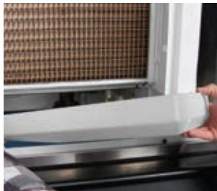
Remove the water reservoir by sliding out, down, and out.
